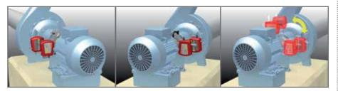
Two measurement points, the 9 and 3 o'clock positions, are all that it takes in order to proceed to live adjustment during the measurement process. The position sensitive detectors measure continuously the misalignment. The large LCD display clearly presents the position of the machinery being aligned. This means no more guessing about the shim amount, or how much to move a machine.
